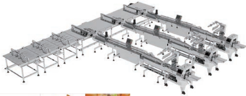
▼ Automated packaging line for cakes with deoxidizer
